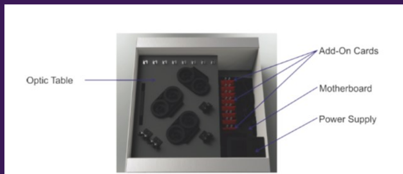
Figure 1. Design concept of Alice's unit in the developed modular QKD setup.
